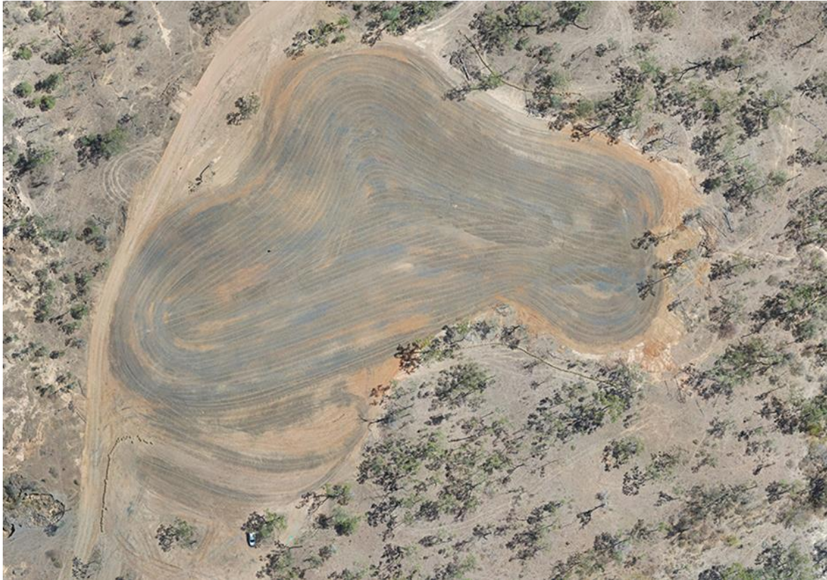
Figure 3: Eroded gully restoration works at Landers Gully, Queensland (Credit: Neilly Engineering Group)
